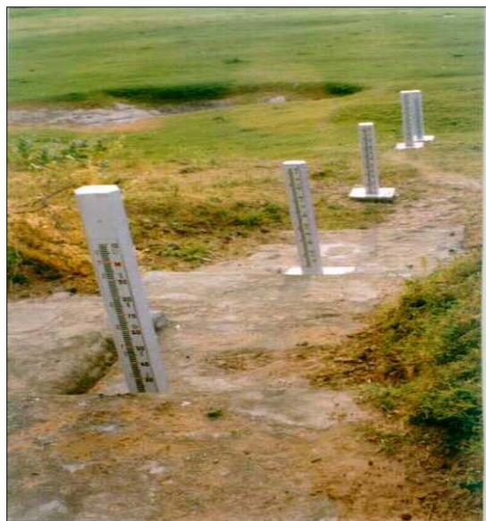
Figure 8.1: Typical Staff Gauge Installation Arrangements
