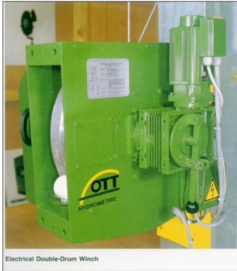
Figure 6.29(c): Unmanned cableway winch (manually operated and electrically operated)
