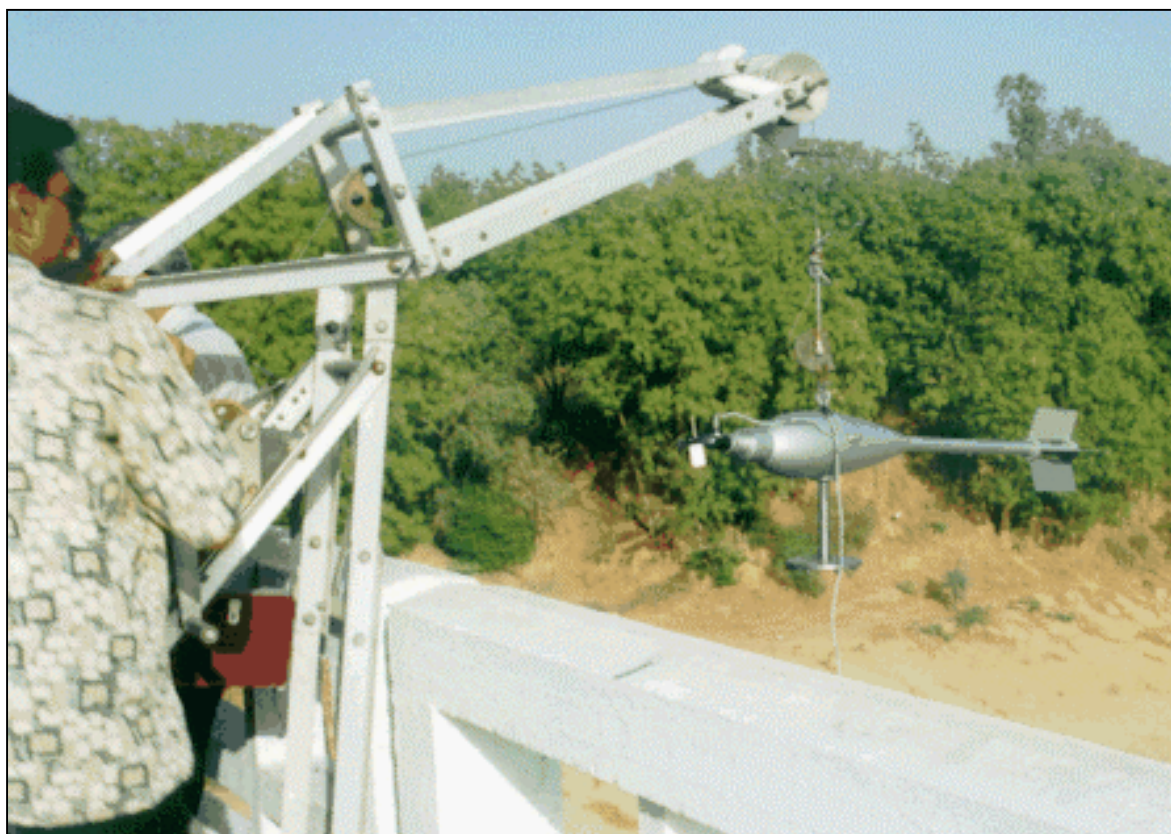
Figure 6.27: Gauging from a Bridge with a Bridge Outfit
