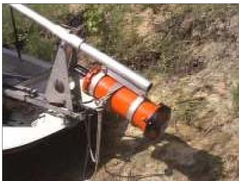
Figure 6.45(b): ADCP deployed from a boat
