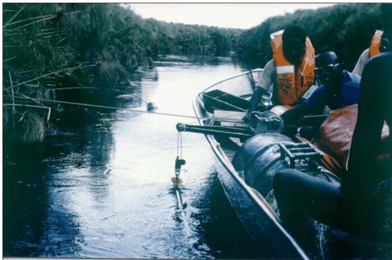
Figure 6.31: Boat gauging using a standard tag line method
